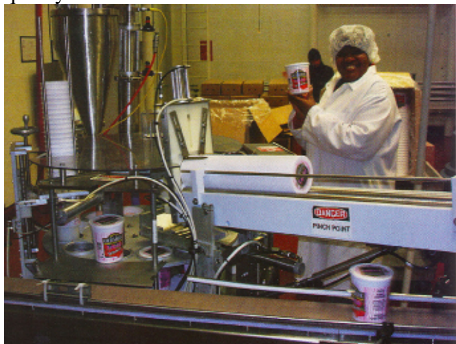
The two cultured product fillers are able to fill yogurt and sour cream in containers ranging from 4 oz to 32 oz.
